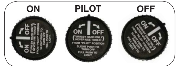
Fig. 21-1 Manual valve operating positions
